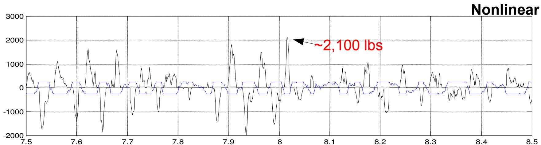
**Battery 5: Shear Force (Node 2183, Zorb) and Relative Displacement – (Blue Line x 40000)
