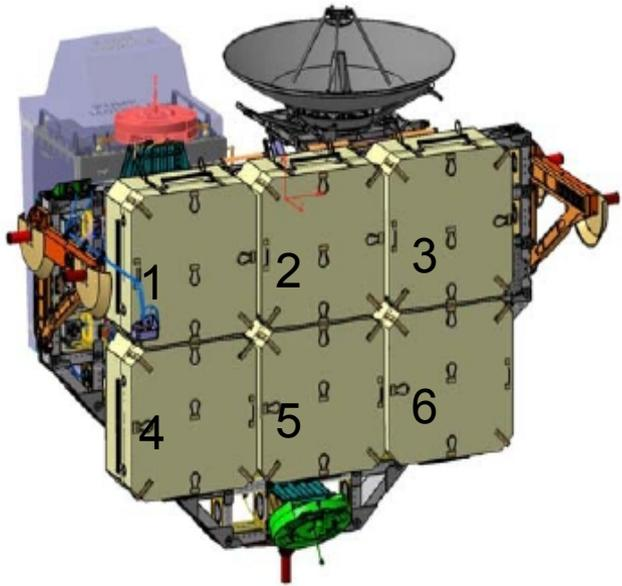
Aft View: 6 Kinematic Mounted Batteries
