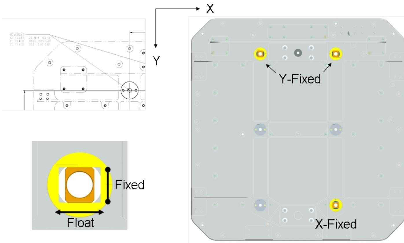
Fixed Shear directions (3 per Battery): **+/- 0.0064"**
