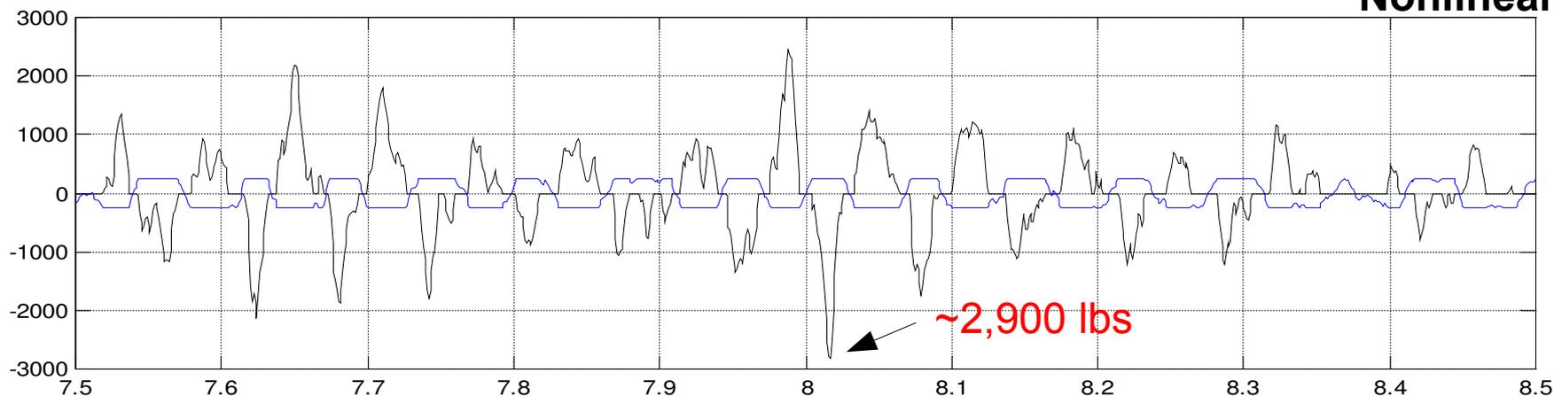
**Battery 5: Shear Force (Node 653, Zorb) and Relative Displacement – (Blue Line x 40000)
