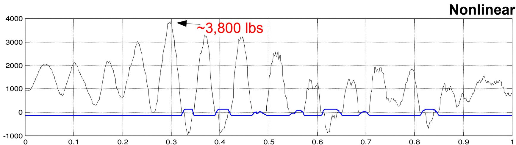
PM: Single Shear Interface Force (Zorb) and Relative Displacement – (Blue Line x 20000)
