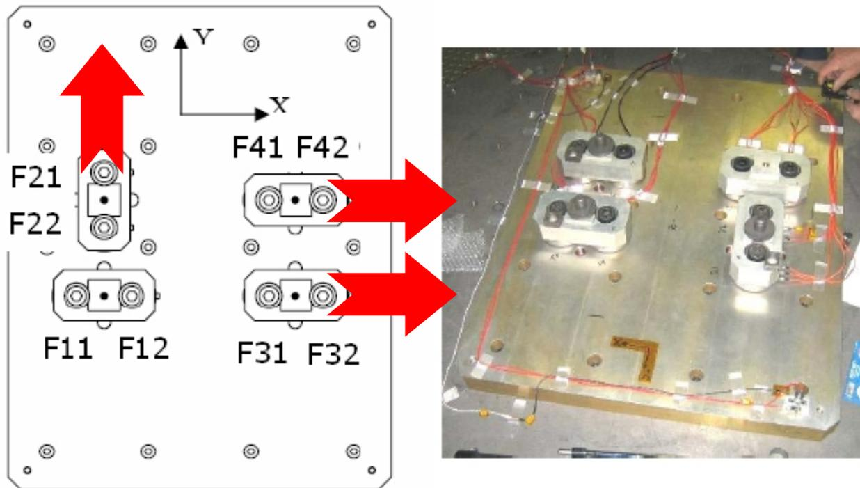
Figure 2-3. Force transducer locations.
